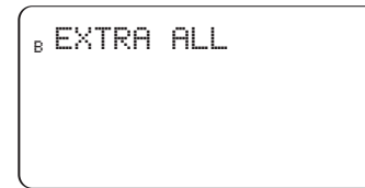
Figure 18: Display showing manual watering, for stations assigned to program B, selected
